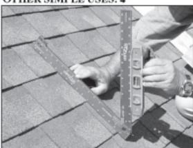
Quickly find an existing pitch by using a level.
