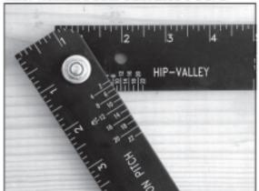
Simply adjust arm edge until it aligns with the desired hip/valley pitch on the scale. The picture above is a 10 hip/valley pitch.
