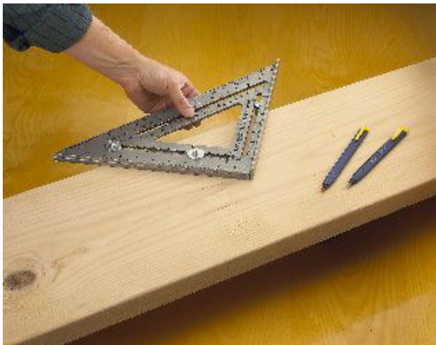
11. Loosen the 2 long hex "stop pegs" from the underside of the square and adjust in the slot for stairway rise and run (tread) measurements.
