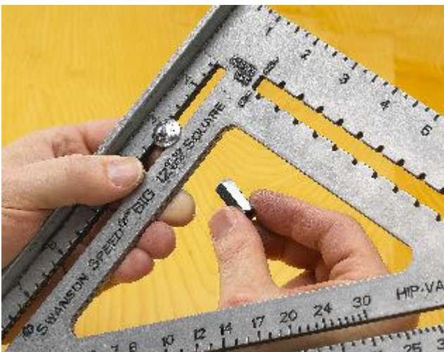
5. With "Big 12®" name on square facing up, place other 1/4"x3/4" bolt through slot next to the words "Big 12®". Thread a washer and hex peg on underside.
