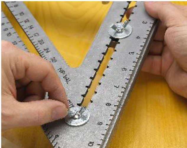
9. Put 2nd smaller bolt up through one ear from underside and through scribe bar slot. Place washer and wing nut on top side.
