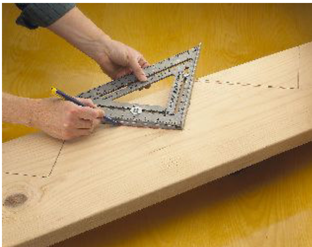
17. Align rise side of square with previously marked rise and re-mark each tread run along Layout Bar.
