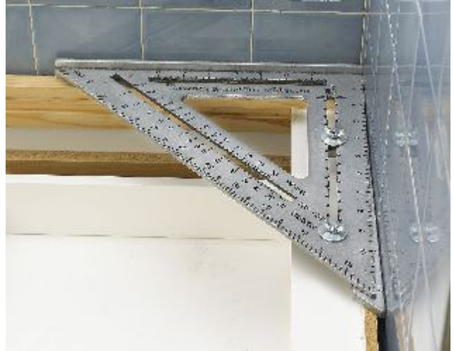
2. SOLUTION: Remove the 2 hex pegs (and bolts) and loosen both Layout Bar wing nuts. Place the Big 12® Speed®Square flush with back wall.
