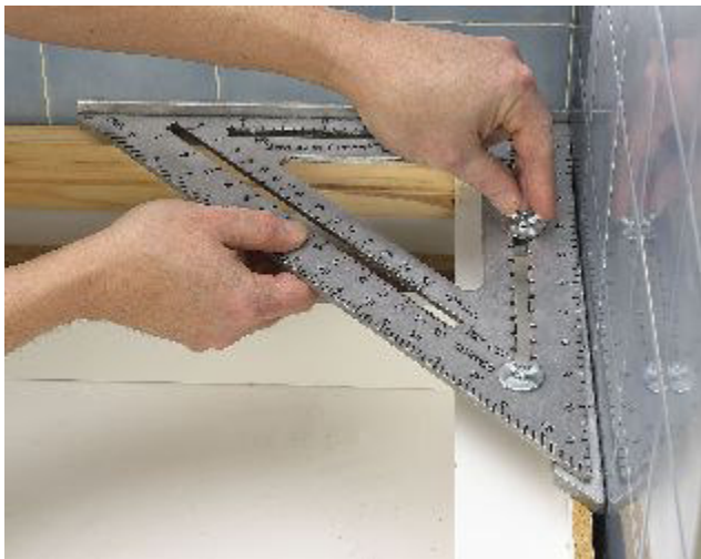
3. While holding the square flat and tight against the back wall, align the Layout Bar flush with the side wall and tighten the rear-most wing nut.
